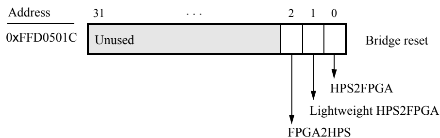
Figure 7. FPGA bridge reset register.
