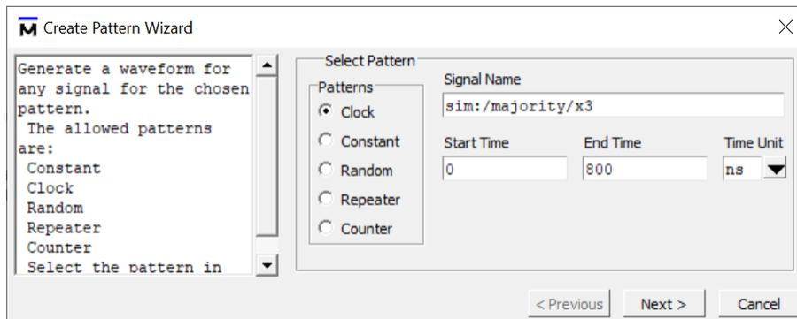
Figure 20. Selecting a signal of clock type.
