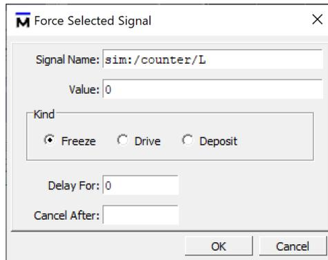
Figure 36. Forcing the *Load* signal to the value 0.
