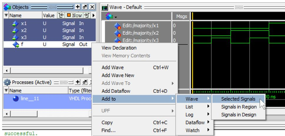
Figure 22. Adding a signal to the Wave window.
