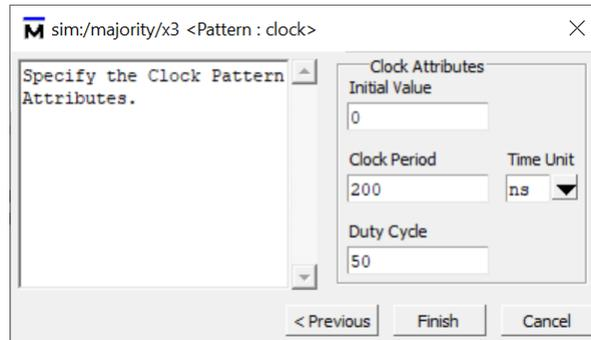
Figure 21. Defining the characteristics of a clock signal.
