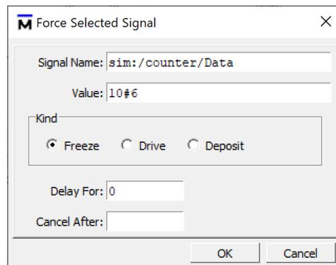
Figure 38. Forcing the value of the *Data* signal..
