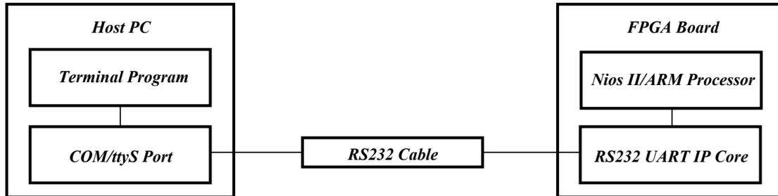
Figure 6. An RS232 UART communication link between the host PC and the FPGA board.
