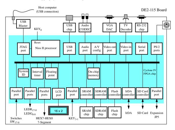
Figure 1. Block diagram of the DE2-115 Computer System.
