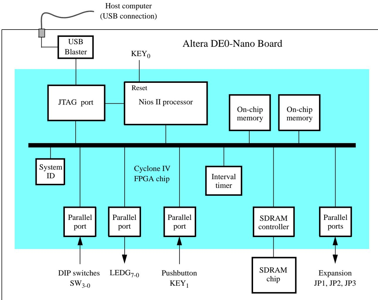
Figure 1. Block diagram of the DE0-Nano Basic Computer.
