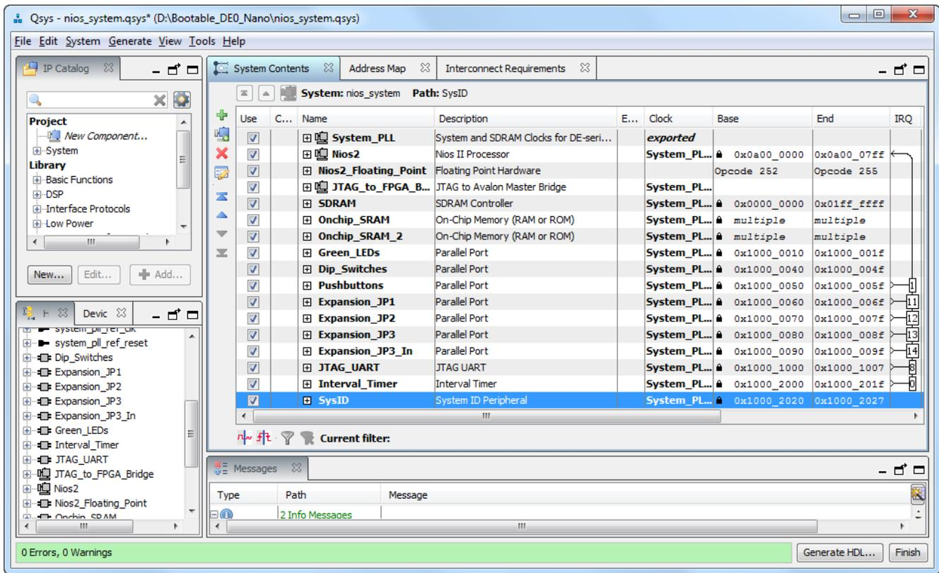
Figure 2. The Platform Designer window for the DE0-Nano Basic Computer.
